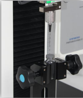
FIXT-NEEDLE-F0217 Rubber Plug Puncture Force Test Fixture
