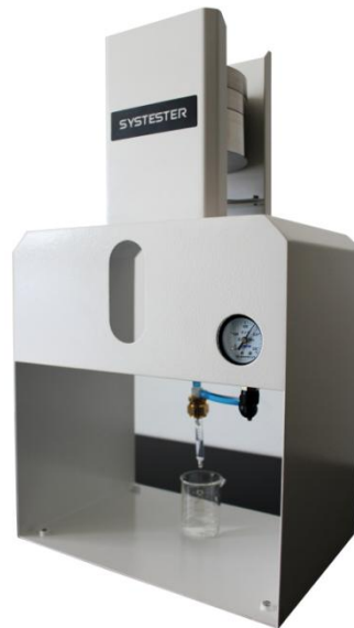
FIXT-CUTT-F0221 Pinhole Patency Test Fixture
