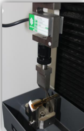
FIXT-NEEDLE-F0217 Rubber Plug Puncture Force Test Fixture
