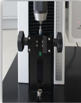
FIXT-PCPO-F0225 Hypodermic Needle and Needle Hub Separation Force Test Fixture
