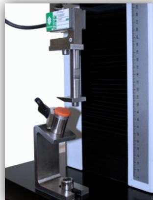
FIXT-INJE-F0215 Piston Sliding Force and Leakage Test Fixture
